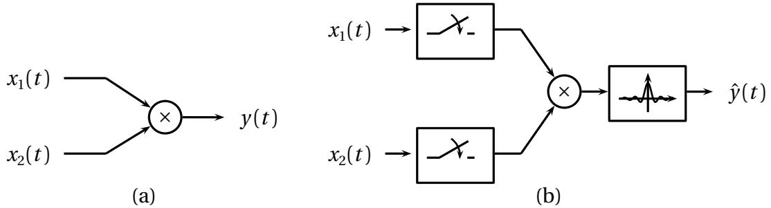
You know that the real-valued, continuous-time input signals are bandlimited, with a maximum positive frequency  $F_N = 8000$  Hz. Determine the minimum value for the rate  $F_s$  so that the discrete-time implementation produces exactly the same output as the continuous-time original system. Explain in detail your choice and, if in doubt, “test” the discrete-time system using the input signals  $x_1(t) = x_2(t) = x(t) = \text{sinc}(2F_N t)$ .
